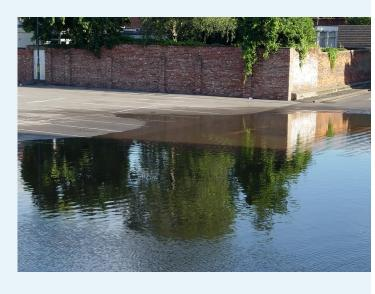
Parking lots are an example of an impervious surface: rain water cannot soak into the ground as it would naturally. To prevent the water from flooding into other areas, including the watershed, catch basins are required to hold and divert the water for treatment.
