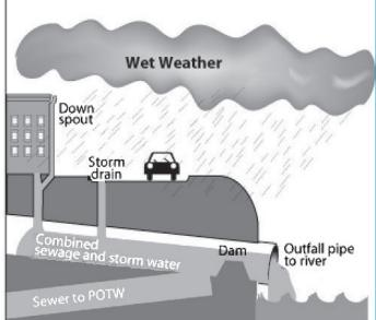
**Combined Sewer** Overflow (CSO): During dry weather (and small storms), all flows are delivered to the publicly owned treatment works (POTW). During large storms, however, some of the combined stormwater and sewage overflows through an "outfall pipe" to an adjacent water body, without proper treatment.
